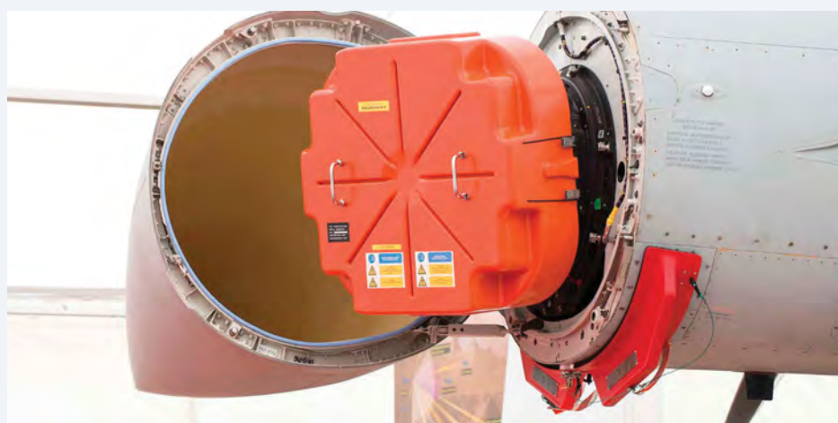
The APG-79 radar of the Super Hornet is typical of older, fixed-antenna AESA radars. Fixed arrays rely entirely on phase shifting to steer the 'beam', and suffer reduced range at higher azimuth and elevation angles Raytheon
