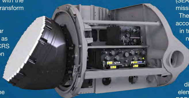
Above: The clearest photo yet of Radar Two, with its innovative single-axis re-positioner, in a representative Typhoon forward fuselage structure Leonardo
