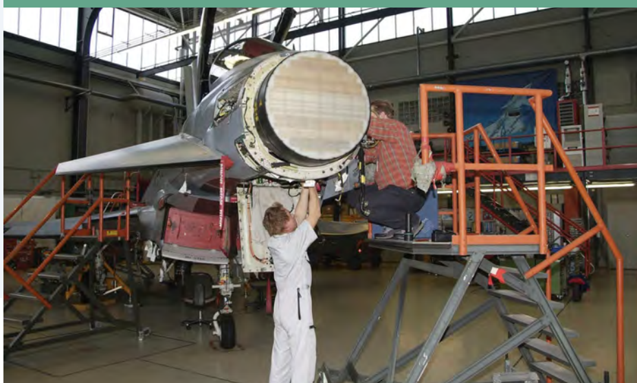
Above: Meggitt has secured a £4.2m contract for the supply of an innovative new nose radome technology to enable effective operation of the ECRS Mk 2 radar. The radome will be tailored to higher and broader bandwidths, but will follow the same outer mould line as the existing item Meggitt. Below: Typhoon's first AESA was the CAESAR (Captor AESA Radar) demonstrator, which flew on board a UK-based BAC One-Eleven, before undergoing a brief series of trials fitted to the German Eurofighter test aircraft DA5. CAESAR had a fixed array. Author's collection
