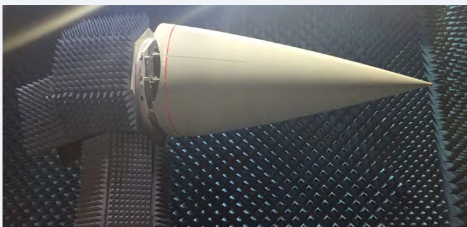
Above: Meggitt has secured a £4.2m contract for the supply of an innovative new nose radome technology to enable effective operation of the ECRS Mk 2 radar. The radome will be tailored to higher and broader bandwidths, but will follow the same outer mould line as the existing item Meggitt. Below: Typhoon's first AESA was the CAESAR (Captor AESA Radar) demonstrator, which flew on board a UK-based BAC One-Eleven, before undergoing a brief series of trials fitted to the German Eurofighter test aircraft DA5. CAESAR had a fixed array. Author's collection
