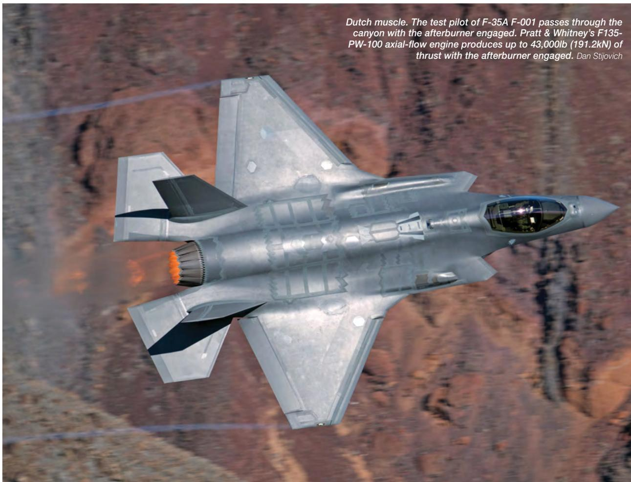
*Dutch muscle. The test pilot of F-35A F-001 passes through the canyon with the afterburner engaged. Pratt & Whitney's F135-PW-100 axial-flow engine produces up to 43,000lb (191.2kN) of thrust with the afterburner engaged. Dan Stijovich*
