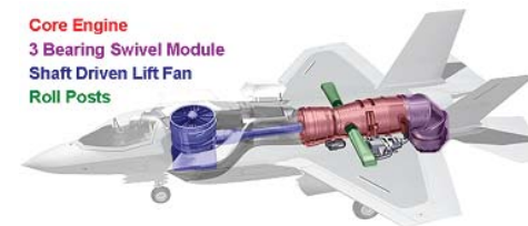
Figure 2. F-35B and its STOVL Propulsion and Lift System.
