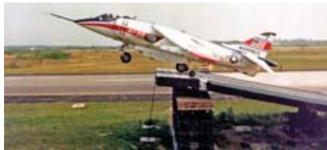
The McDonnell Douglas AV-8 Harrier was tested on a 12-degree ski jump for suitability on small-deck carriers in July 1979. It was flown by Capt. Russ Stromberg, USMC.
