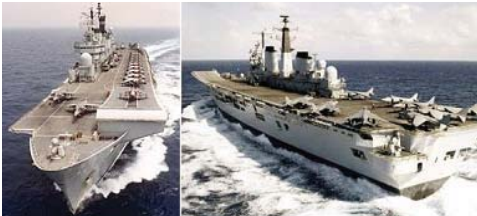
Figure 4. HMS Illustrious with retrofitted 12° ramp.
