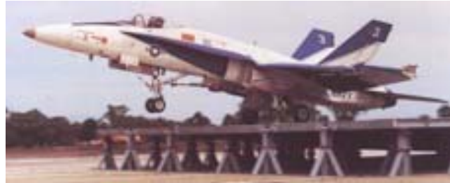
The McDonnell F/A-18A first flew from a ski jump on 26 September 1983. It flew 91 ski jump tests at ramp angles of 6- and 9-degrees and achieved takeoff distance reductions of 66%.
