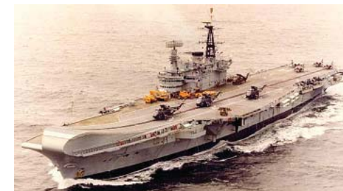
Figure 3. HMS Hermes with first 12° ski jump ramp.
