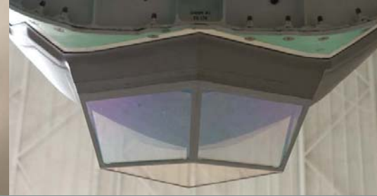
System: AN/AAQ-40 Electro-Optical Targeting System. Detail: The aft end of the faceted window assembly showing three of the seven sapphire panels. Photograph: Lockheed Martin
