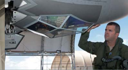
System: AN/AAQ-40 Electro-Optical Targeting System. Detail: The faceted window of the EOTS on an F-35A assigned to the 58th Fighter Squadron based at Eglin Air Force Base, Florida. Photographer: Jim Haselaine
