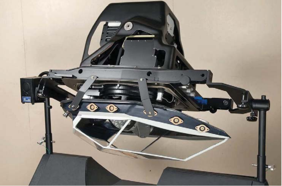
ABOVE: The EOTS measures approximately 19.4 x 27.5 x 32.1 inches (493 x 698 x 815mm), weighs 202lb (91kg) and populates a box with a volume of less than 4ft³. LOCKHEED MARTIN
