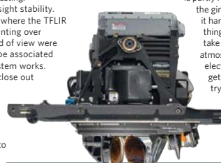
System: AN/AAQ-40 Electro-Optical Targeting System. Detail: The local and elevation assemblies of the EOTS. Photograph: Lockheed Martin
