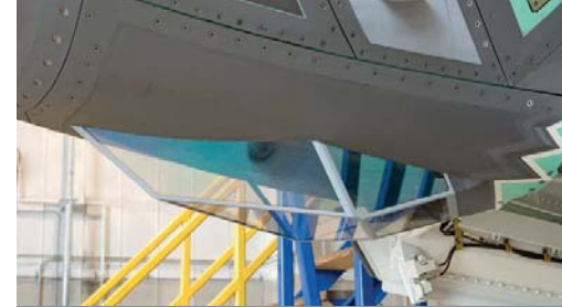
System: AN/AAQ-40 Electro-Optical Targeting System. Detail: The sapphire colour of the panels is shown to good effect in this side shot of the EOTS faceted window. Photograph: Lockheed Martin
