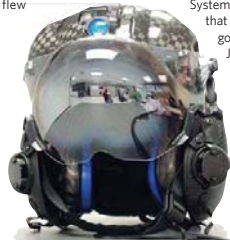
System: Gen III Helmet-Mounted Display Detail: The upgraded Gen III HMD fitted with an ISIE-11 camera Photograph: Rockwell Collins
