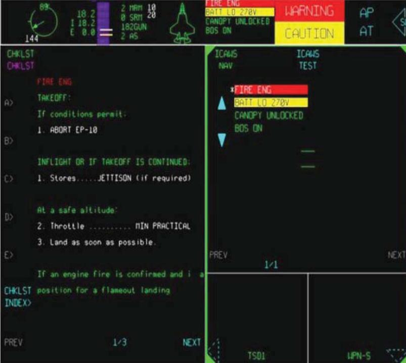
Figure 8. Integrated Caution and Warning System (ICAWS)
