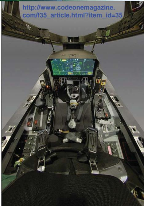
With stealth, fully integrated avionics, advanced sensor fusion, and a dizzying array of interoperability and data-exchange requirements, the F-35 Joint Strike Fighter represents more revolution than evolution. Nowhere are the advances in this multireole combat fighter more starkly illustrated than in the cockpit.
