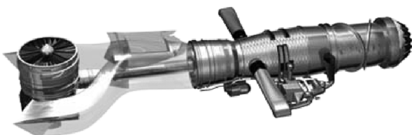
Fig. 3 Shaft-driven lift fan propulsion system.
