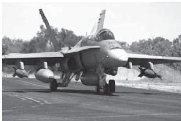
An RAAF 'Classic Hornet' with two 2,000lb laser guided bombs and two long range fuel tanks taxiing out for a bombing sortie. Land based aircraft will always be far from the amphibious operation and waste time and fuel to transit to and fro. Added to this is the time to rearm and pilot rest. Having CAS assets much closer saves time, pilot fatigue and money, as well as a better capability outcome.
