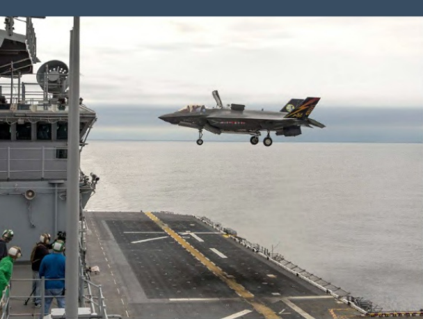
An F-35B hovers over an area of flight deck coated with the new Thermion heat-resistant deck coating during trials on USS Wasp in August 2013.
