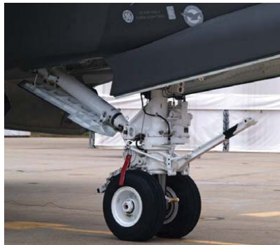
Below: The CV nose gear staged shock strut carries a very complex mechanism to position the launch bar on to the catapult. Kin - Max Irons Opposite: Landing gears for the F-35C CV variant are unique and differ to the F-35A and F-35B systems to withstand the extreme high energy landings typical of naval aircraft operating from an aircraft carrier. Lockheed Martin
