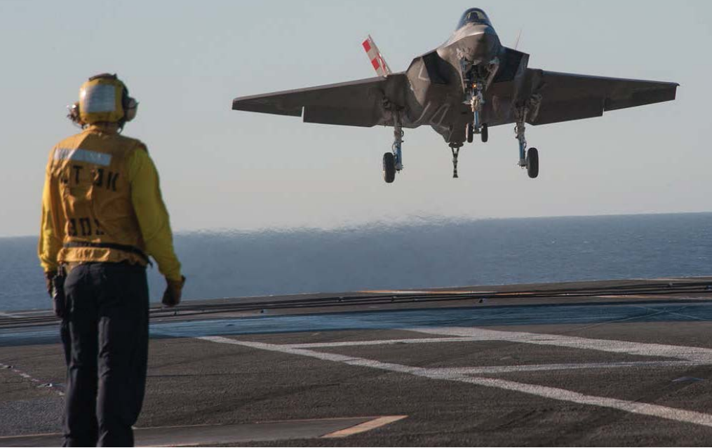
Above: CF-05 lands aboard the USS Nimitz during the initial shipboard trials. The F-35C performed its first set of arrested landings and catapult launches
