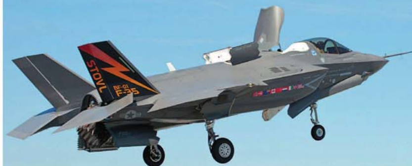
Balancing the thrust of the engine-driven LiftFan in vertical flight, the segmented tailpipe curves to deflect jet exhaust downwards
