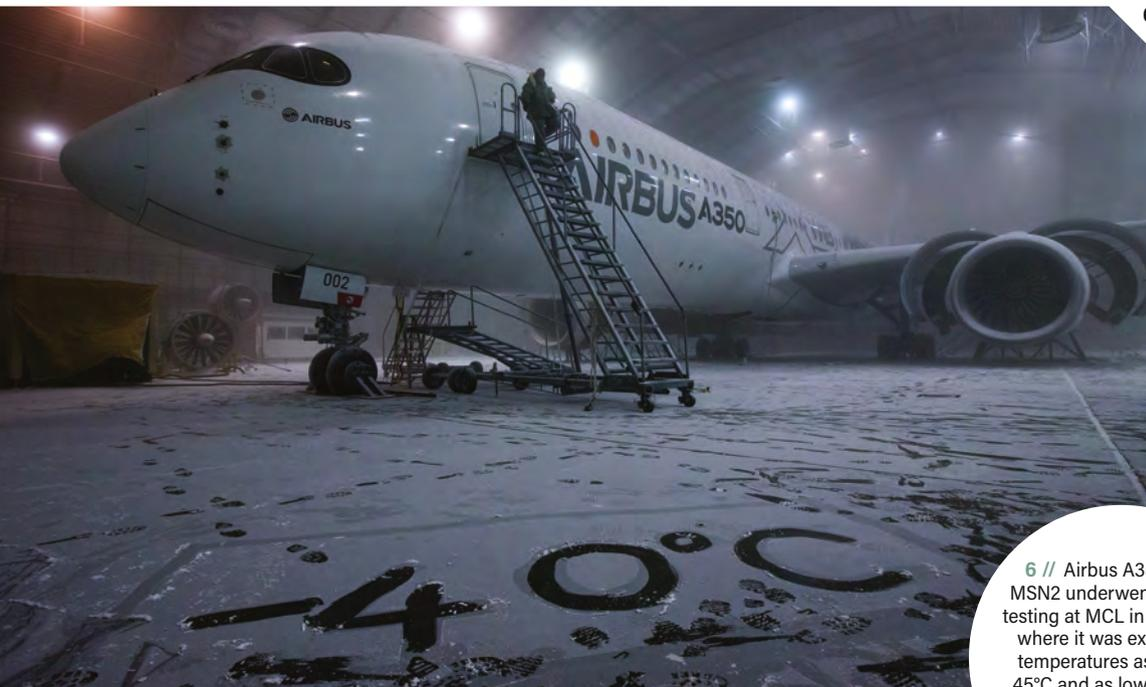
6 // Airbus A350 XWB MSN2 underwent climatic testing at MCL in June 2014, where it was exposed to temperatures as high as 45°C and as low as -40°C
