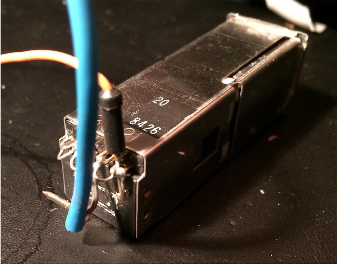
NO stands for "Normally Open", thus does not supply power when the relay is open (not activated by Pokeys). This is what you want to connect when your indicator should be off unless given a signal. NC stands for "Normally Closed", thus supplies power until the relay is closed.
