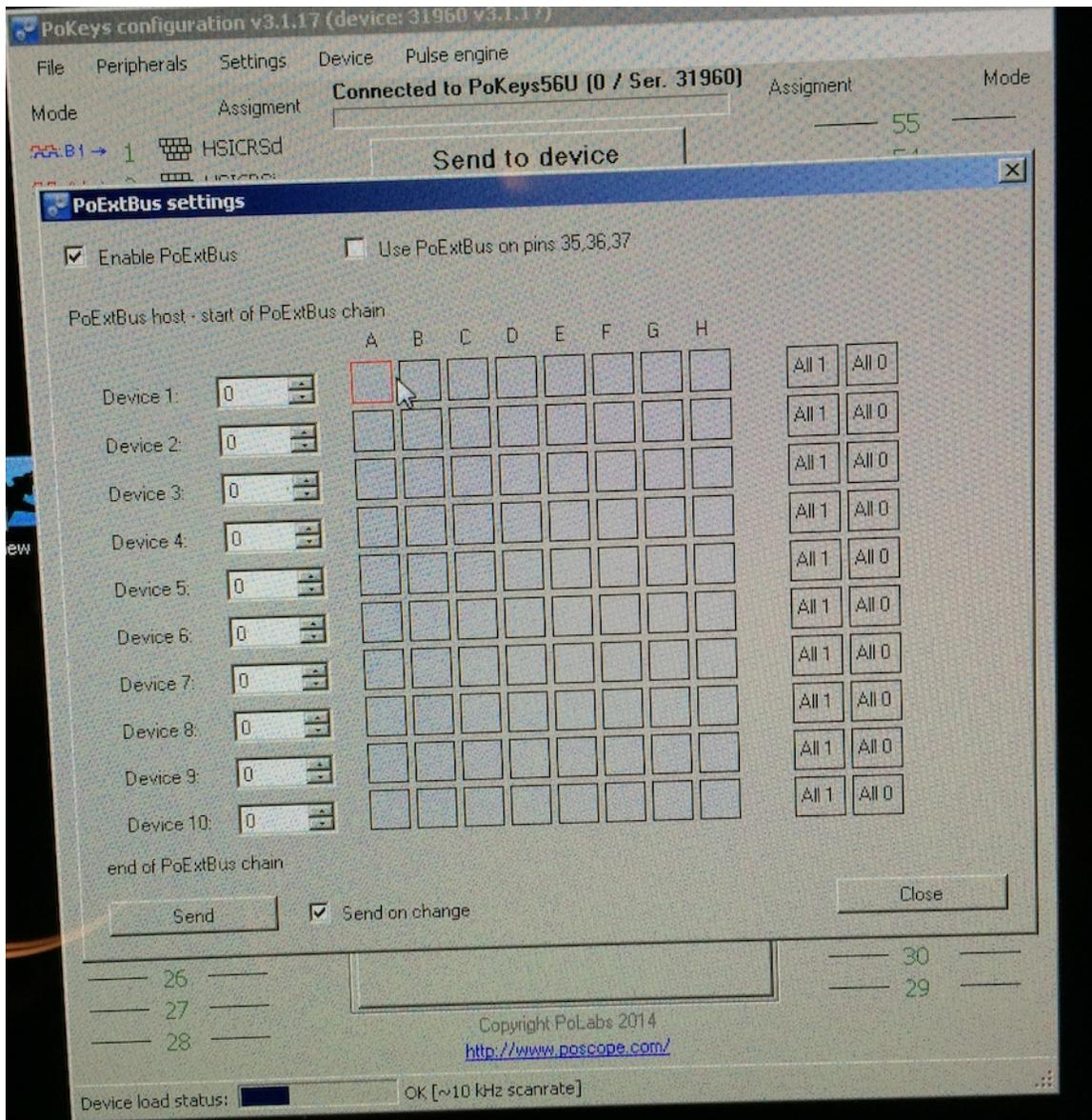
To test, it's easier to check the box on the bottom "send on change" so you don't need to hit the big 'send' button each time. If you left click on a square, it lights up green and you should hear the relay close on the board. A yellow-orange led lights up to indicate the relay is closed on that side.
