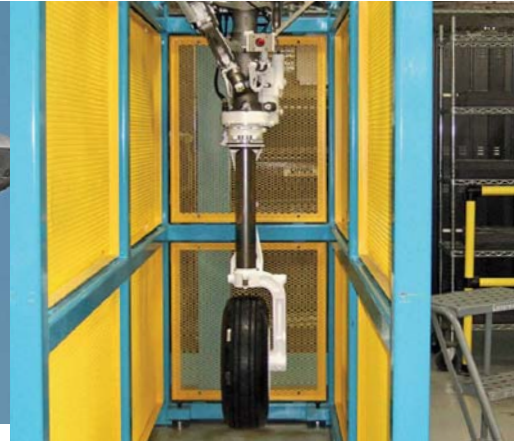
An F-35A CTOL nose gear in a test jig. GOODRICH
