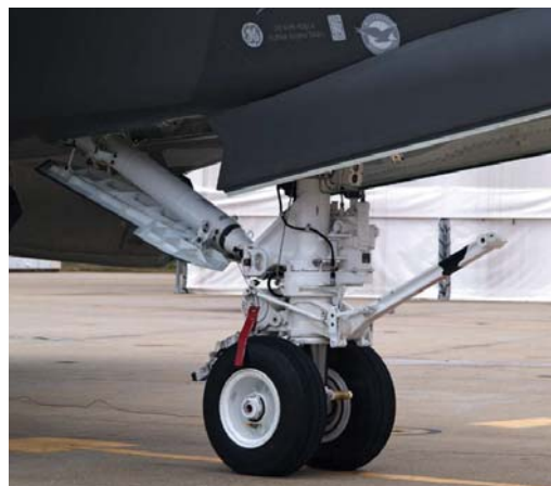
ABOVE: The CV nose gear staged shock strut carries a very complex mechanism to position the launch bar on to the catapult. KEY - MARK AYTON
