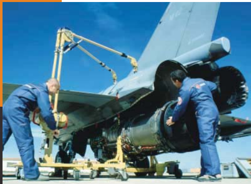
Thanks to its advanced conception, the M88 can be replaced in under an hour.
