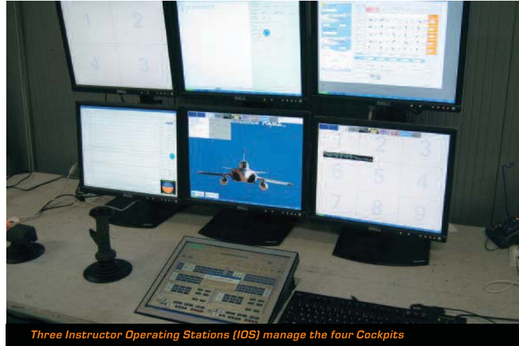
Three Instructor Operating Stations (IOS) manage the four Cockpits
