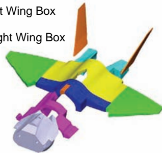
Plate 2 Joint strike fighter fuel tank layout (Courtesy of BAE Systems) (See Figure 3.10) http://www.mecatronica.eesc.usp.br/wiki/upload/f/fa/2008_OK_Aircraft_Systems.pdf
