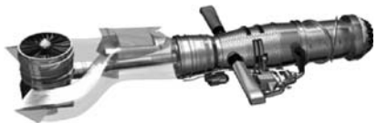
Fig. 3 Shaft-driven lift fan propulsion system.
