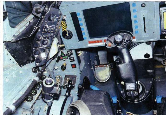
VAAC work will lead to the deletion of the nozzle control lever (inboard of the throttle)
